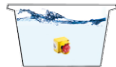
IP67: Submersion to one meter for 30 minutes.
